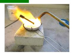
A new melting dish or crucible must be given a protective coating of borax before its first use. Borax extends the life of the ceramic material. Once done, it generally does not have to be repeated.
